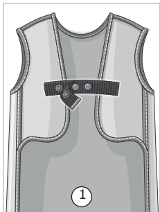
Press-stud closure Elastic band with press stud for closing at the back.
